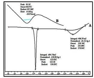
Figure 3. DSC thermogram of (A) Pure drug Rosuvastatin, (B) Liquisolid powder system (F3).
