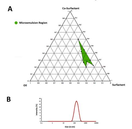
Figure 2. The pseudo-ternary phase diagram (A) constructed by ProSim software for a mixture of castor oil, Cremophor RH60, and PEG1500 respectively as oil, surfactant, and co-surfactant. Size distribution (B) of formulations investigated by a zeta-sizer at 25°C
