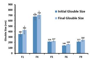
**Figure 3.** The Globule size changes of F1, F4, F5, F6, and F9 formulations after three replicates of freeze-thaw cycles with 48 h incubation at each temperature (-20 to +25 °C) during the stability test
