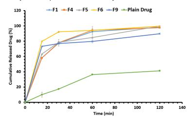
Figure 5. In vitro release profiles of different SMEDDS formulations along with the plain drug estimated by the dissolution test in USP type II apparatus filled with HCI 0.1 N at 37°C
