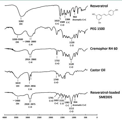
Figure 4. FTIR Spectra of resveratrol, PEG<sub>1500</sub>, Cremophor® RH60, castor oil, and solidified SMEDDS
