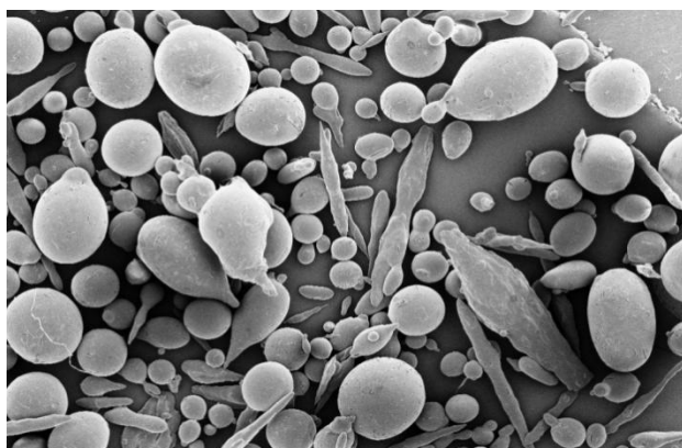
Figure 1. SEM of a spherical microspheres containing anhydrous theophylline F 5 (drug: polymer ratio 1:6) at 50x.
