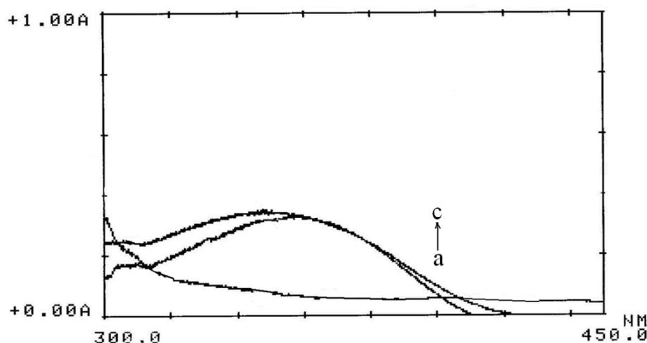
**Figure 7.** Absorption spectra of (a) urine blank, (b) Standard solution of PX (1.8 µg/mL) (c) collected urine after oral administration of 10 mg of PX and β-glucuronidase treatment; other conditions have been mentioned in Figure 2.
