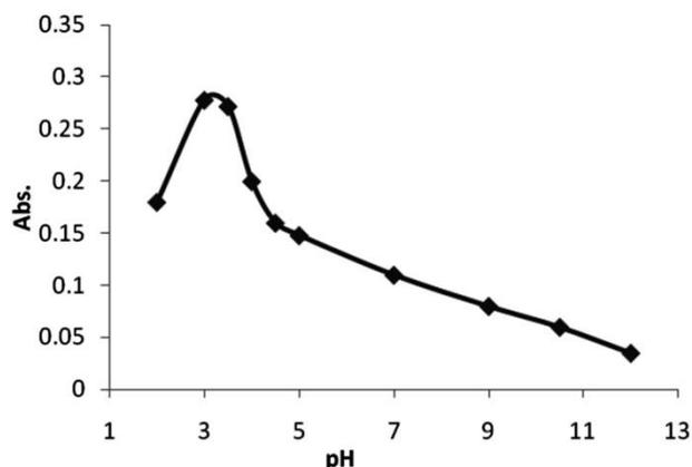
**Figure 2.** Effect of pH on the analytical responses, PX (1.2 µg/mL); other conditions: 2.0 mL of 20% NaCl; 0.5 mL of 1.0 mol/L acetate buffer at pH 3.0; extraction with 500 of methanol µL containing 50 µL of chloroform.
