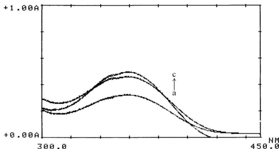
**Figure 1.** Absorption spectra of PX after DLLME: a) Standard solution of PX (2.0 µg/mL) (b) sample "a" after addition of NaCl (8% w/v), (c) 0.5 mL urine sample spiked with PX (2.0 µg/mL); other conditions: 0.5 mL of 1.0 mol/L acetate buffer at pH 3.0; extraction with 500 of methanol µL containing 50 µL of chloroform.
