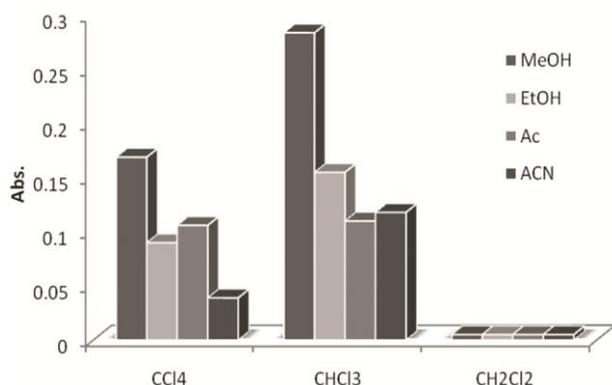
**Figure 3.** Effect of the type of extraction and dispersant solvents on the analytical responses, EtOH: ethanol, MeOH: methanol, Ac: acetone, ACN: Acetonitrile, PX (1.8  $\mu\text{g/mL}$ ); other conditions have been mentioned in Figure 2.
