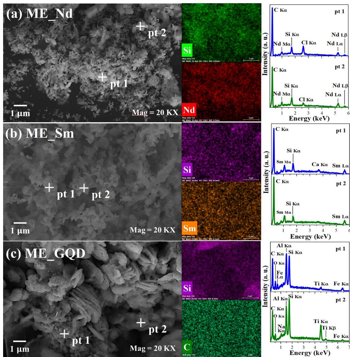
**Figure 1.** Micrographs, compositional maps, and EDS line spectra were obtained from the points (pt) indicated in the micrographs of the nanoparticles (a) ME\_Nd, (b) ME\_Sm, and (c) ME\_GQD. The identified elements were silicon (Si), neodymium (Nd), samarium (Sm), carbon (C), chlorine (Cl), calcium (Ca), oxygen (O), iron (Fe), aluminum (Al) and titanium (Ti).
