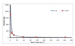
Figure 2. A sample viscosity curve for formulated suspension
