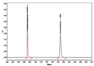
**Figure 2.** UPLC overlay chromatogram of Losartan Potassium and Chlorthalidone
