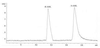
**Figure 2.** Capillary electrophoretic separation of AML enantiomers using RAMEB as chiral selector (experimental conditions: BGE: 25mM phosphate buffer, chiral selector: 20 mM RAMEB, pH - 3.0, voltage + 25 kV, temperature 15°C, hydrodynamic injection 50 mbar/1 sec., sample concentration 10  $\mu$ g/ml, UV detection 238 nm)
