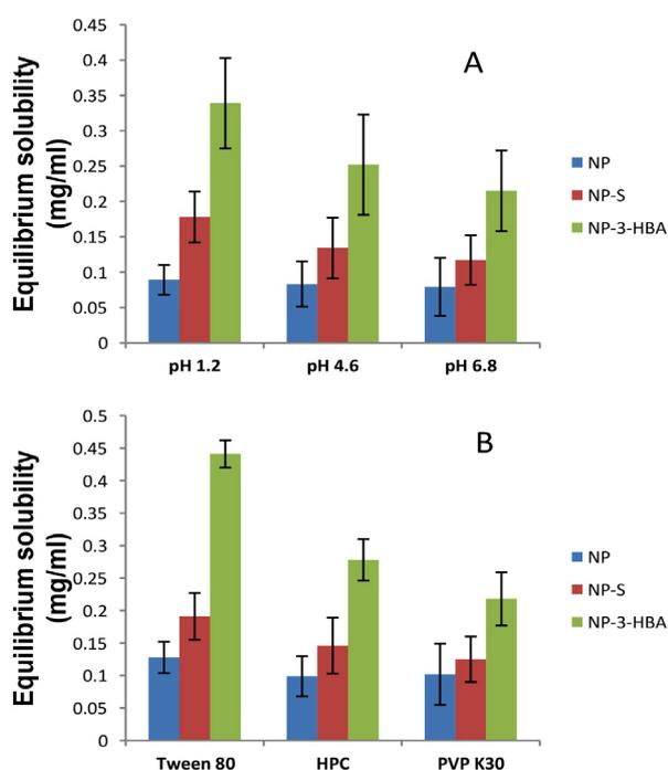
**Figure 3.** Effect of pH (A) and surfactant (B) on equilibrium solubility of NP (nevirapine), NP-S (nevirapine-salicylamide cocrystal), NP-3-HBA (nevirapine-3-hydroxy benzoic acid cocrystal).
