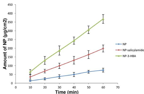
**Figure 4.** Dissolution profiles of NP-nevirapine, NP-S: nevirapine-salicylamide cocrystal, NP-3-HBA:nevirapine 3-hydroxy benzoic acid cocrystal.
