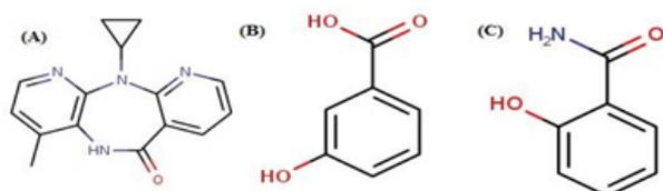
**Scheme 1.** Structure of nevirapine (A), 3-Hydroxy benzoic acid (B), Salicylamide (C).
