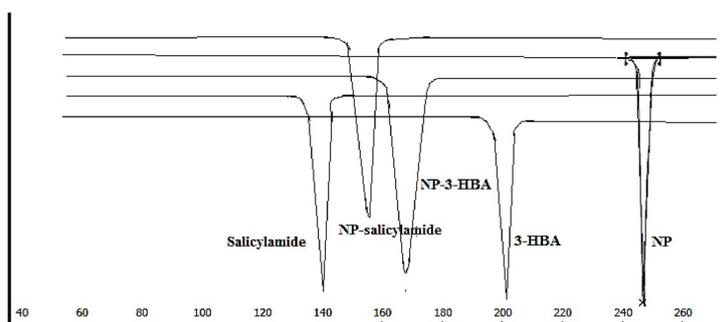
**Figure 1.** DSC thermograms of NP (nevirapine), 3-HBA (3-hydroxybenzoic acid), Salicylamide, NP-3-HBA (nevirapine-3-hydroxy benzoic acid cocrystal), NP-salicylamide (nevirapine-salicylamide cocrystal).
